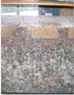
Model of aggregate layers for stability and detention capacity. Photo by Michelle DeLaria.
