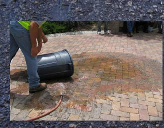
that was installed outside of their office building last fall. Staff showed our group the "barrel test" that is common at permeable pavement sites. This is when a 30 gallon barrel is filled with water and dumped on the pavement so people can see that the water rapidly infiltrates into the surface of the permeable pavement instead of flowing across the surface.
